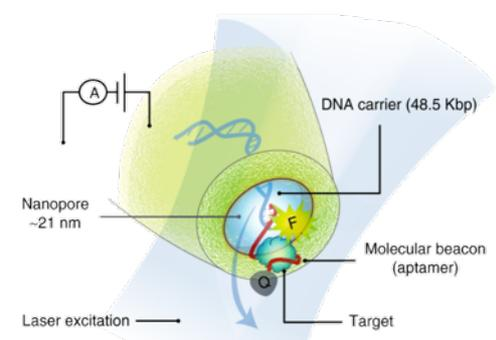
**Figure 1** | Schematic of the electro-optical configuration where a nanopore is integrated with a single-molecule fluorescence confocal microscope.
